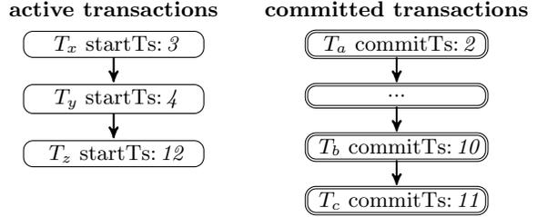
Figure 4: **Transaction lists** – Ordered for fast GC
