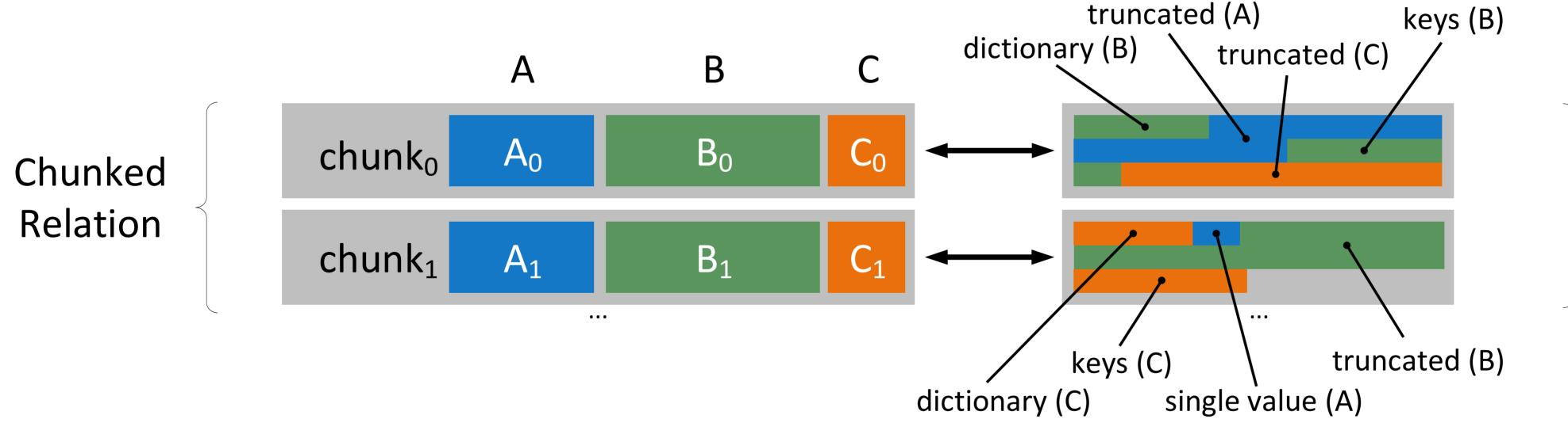
Cold chunks are transformed into individually compressed Data Blocks
