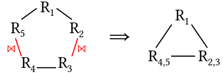
Figure 6: Pentagon query transformed into a triangle query
