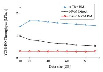
**Figure 14: Large Workloads** – YCSB-RO point lookup performance for large workload sizes. The NVM capacity is configured to match the data size, and the DRAM capacity is set to a fifth of that of NVM.
