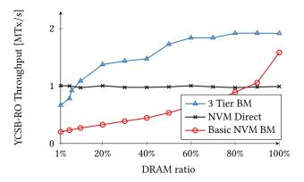
Figure 13: DRAM Buffer Size – YCSB-RO performance for varying amounts of DRAM and a fixed NVM capacity (YCSB with 10 GB of data, read only and 10 GB NVM).
