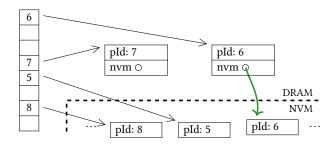
**Figure 7: Single-Table Mapping** – Using one hash table for DRAM and NVM-resident pages eliminates most overhead for managing the SSD layer. The hash table entries are identified by their location in memory (DRAM or NVM).
