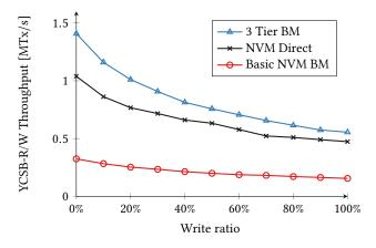
**Figure 15: Update Performance** – YCSB-R/W performance with an increasing amount of write transactions (YCSB with 10 GB of data, 2 GB DRAM, and 10 GB NVM).
