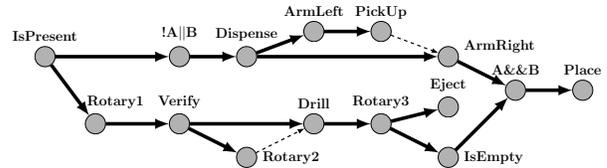
(c) Advanced version of the previous workflow that runs the distribution and processing stations in parallel
