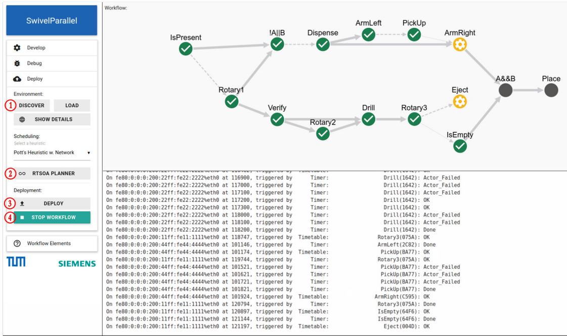
Fig. 7: Screenshot of the graphical user interface for the rtSOA demonstrator. After generating and deploying a service choreography by pressing the buttons marked 1-3, the user has started the execution of the workflow with the button marked by the number 4. The system is currently executing the workflow and the GUI is displaying a live visualization of the system state. A video showing the process described here can be found at <https://youtu.be/SaXwwf0m65I>
