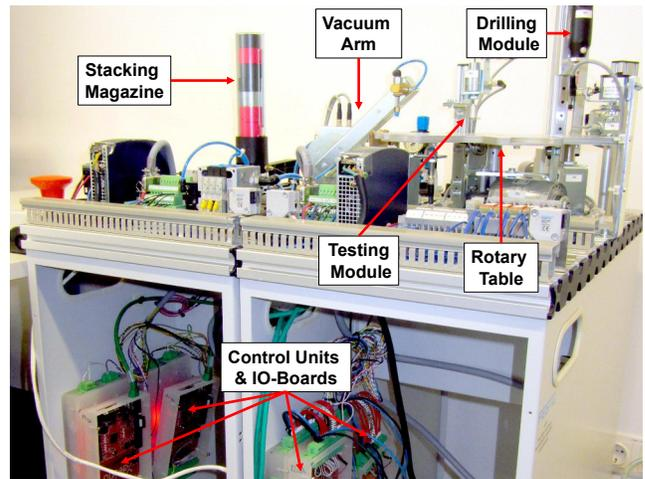
Fig. 3: The demonstrator consists of a Festo MPS distribution station and processing station, controlled by five Olimex STM32-P107 development boards
