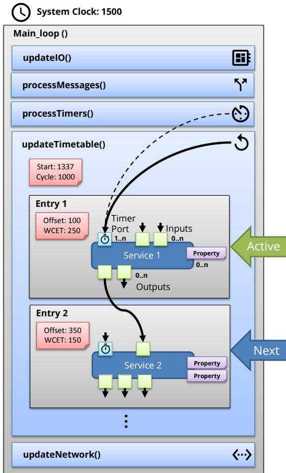
Fig. 4: Illustration of the main loop on the nodes controlling the demonstrator. The `updateTimetable()` method is the central control point in this time triggered system as it triggers the execution of all scheduled service instances on the node.
