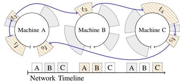
Fig. 1: Devices cooperating in a distributed service choreography follow local cyclic schedules and communicate over a real-time TDMA network. Hatched areas indicate resources used by an example workflow, arrows represent data flow.
