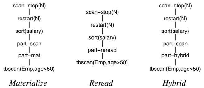
Figure 3: Range Partitioning Plans for Query 1
