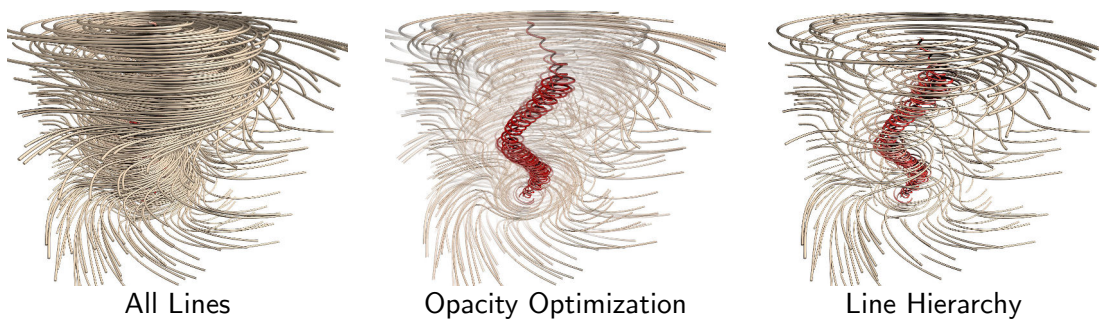
Figure 1.6.: Comparison of different state of the art methods with an unfiltered image. The middle image shows opacity optimization by Günter [GRT13], the left adaptive line hierarchy by Kanzler [Kan16]. Curvature is used as relevance criterium. (Figure adapted from [Kan16])
