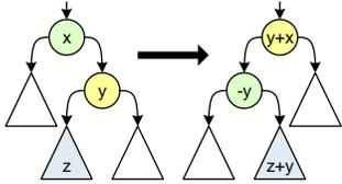
Figure 8: Left rotation in the accumulation tree
