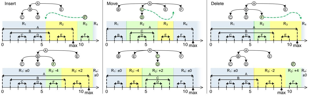
**Figure 2: Updating a hierarchy with  $insertBefore(6)$  (left),  $moveSiblingRangeBefore(C, C, 9)$  (middle), and  $deleteSiblingRange(F, F)$  (right). These operations are modeled by swapping  $R_2$  with  $R_3$  and updating  $max$ .**
