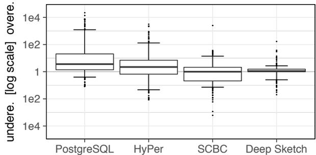
**Figure 3: Estimation errors on the query workload. The box boundaries are at the 25th/75th percentiles and the horizontal “whisker” lines mark the 95th percentiles.**
