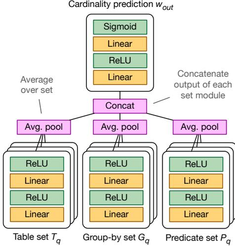
**Figure 2: Architecture of our MSCN model. Tables, group-by columns, and predicates are represented as separate MLP modules that provide input to a final output network that predicts query cardinalities.**
