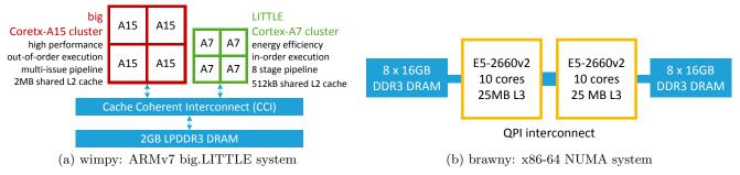
Figure 2: Demonstration platforms: (a) a wimpy smartphone system and (b) a brawny server system
