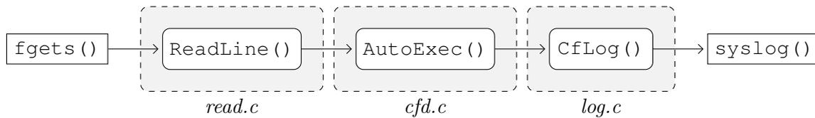
Figure 8.8.: Data flow causing the format string vulnerability in *CFEngine 1.5.x*.
