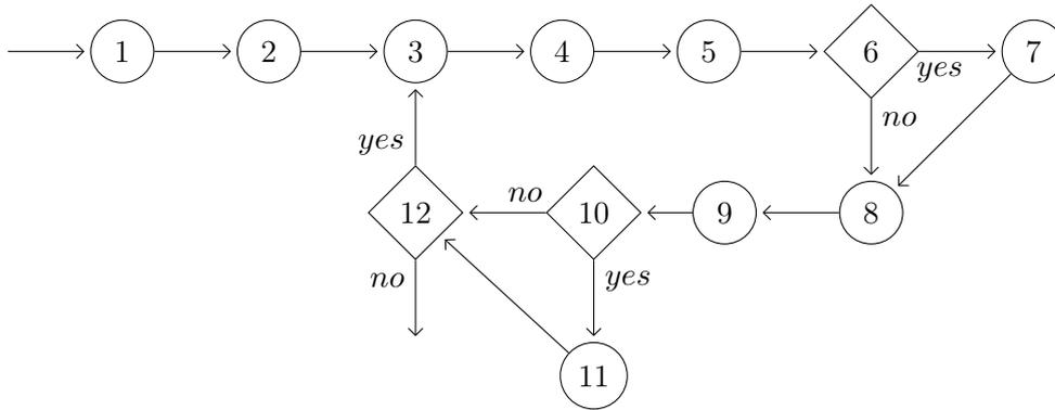
Figure 6.1.: CFG with node numbers that correspond to the line numbers in Listing 6.1.
