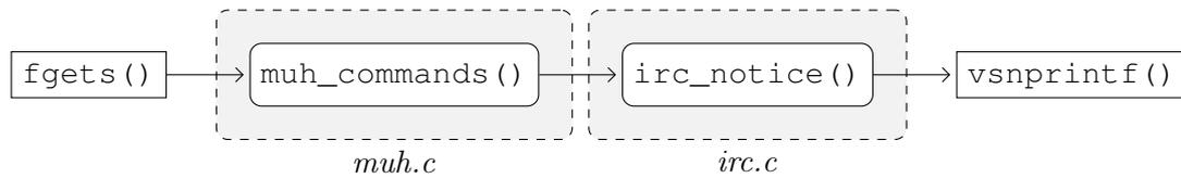
Figure 8.6.: Data flow causing the format string vulnerability in *muh 2.0.5c*.
