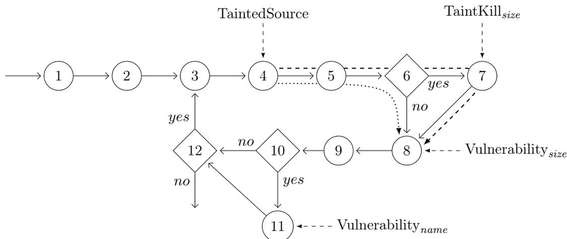
Figure 6.4.: CFG with a valid (dotted) and a spurious (dashed) path to  $Vulnerability_{size}$ .
