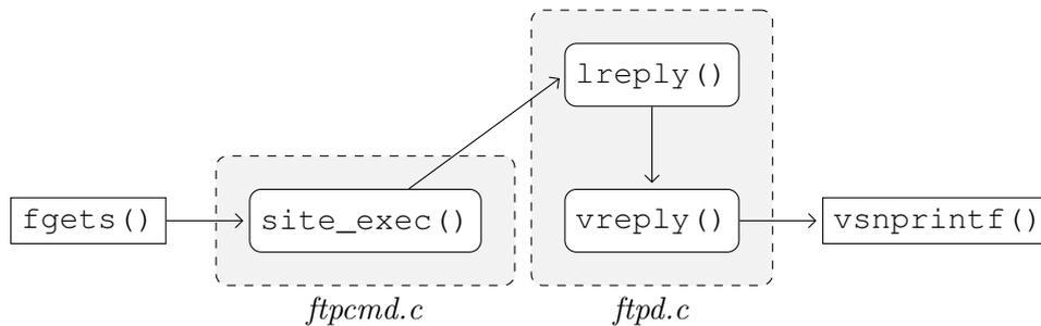
Figure 8.7.: Data flow causing the format string vulnerability in *wu-ftpd 2.6.0*.
