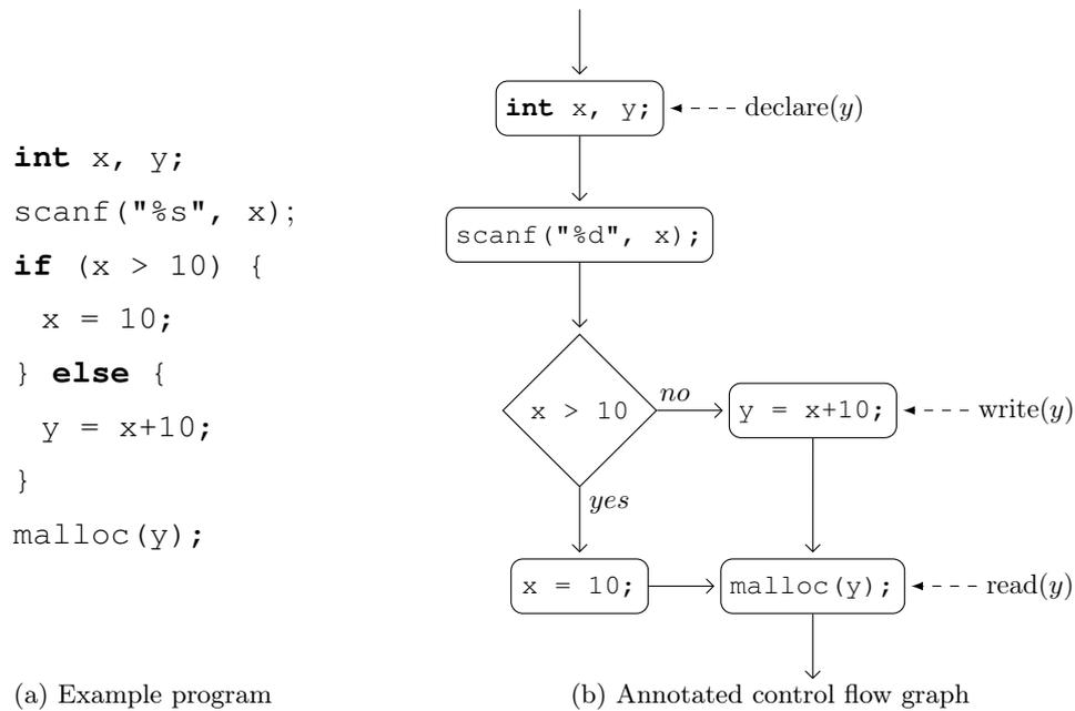
Figure 4.6.: Example program and its annotated CFG for the write-before-read property.
