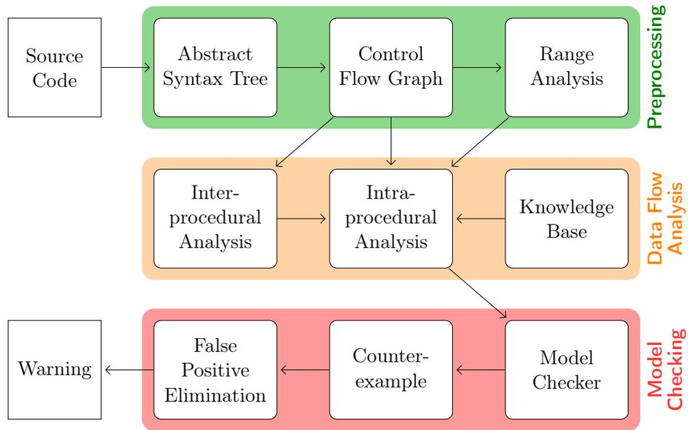
Figure 5.1.: Architecture of the taint analysis embedded in the Goanna model checker.
